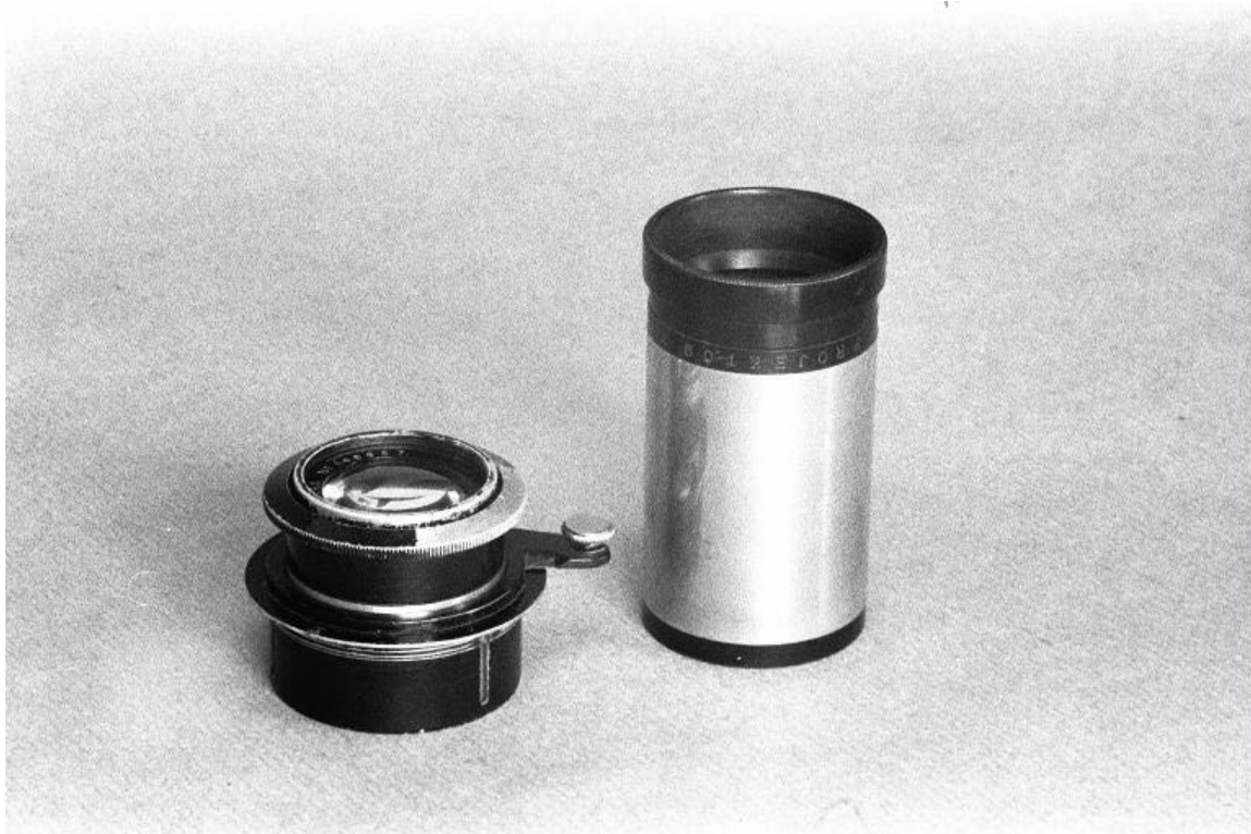
Fig 004 027 Voigtlaender f4.5 Heliar (apparently a 4-glass type) and Projektos projection lens, fc.3 12cm No116,970.
