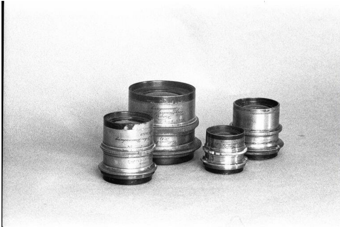
Fig 004 009 Voigtlaender Kollinear (l) f6.3 at Nos 54,85x (1899) and 46,370 (1895);(r) f5.4 at Nos 54,37x and 117,67x.
