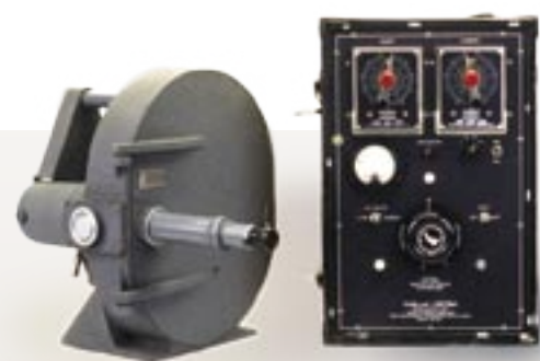
142 Fastax 8mm camera and the "Goose" camera control unit used by Dr. Harold Edgerton to photograph atomic bomb test of November 1, 1952, at speeds up to 16,000 images per second.
